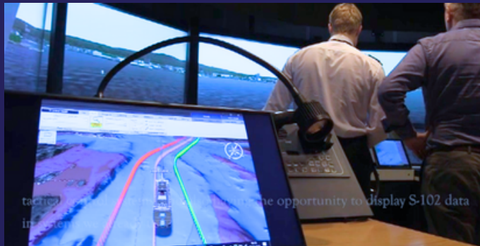
Testing of S-102 depth data in a Kongsberg Bridge Simulator
